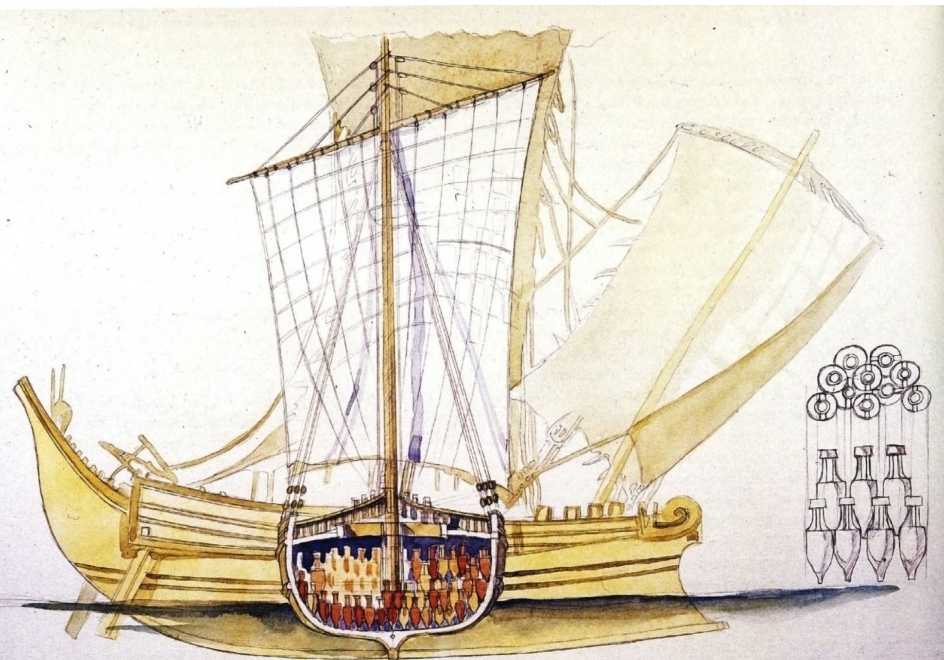
Roman ship Roman ship showing stowed amphoras, after the Madrague de Giens shipwreck, dated 75 to 60 BC, estimated dimensions 40 x 9 m and 3.5 m draught for 375 ton of cargo (by Jean-Marie Gassend, 2005)
